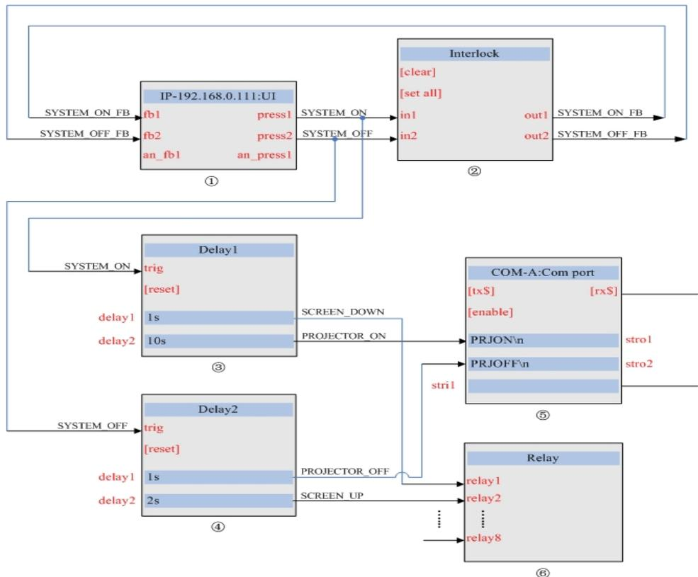
The above diagram shows a simple testing program compiled with the “Logic Master” software. Refer to help documents of the “Logic Master” software for more information.
