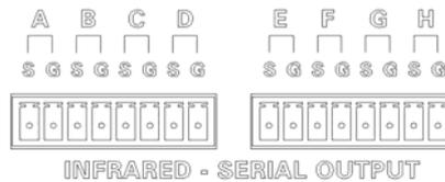
Each one of the eight ports may serve as an IR output or one-way RS-232 output. S is signal Positive and G is GND. The carrier frequency of IR output is up to 1.2MHz and data transmission rate 115K/s. The amplitude of the output via the one-way RS-232 port is the level of TTL, i.e. 0 to +5V. This is likely inapplicable to control some devices.
