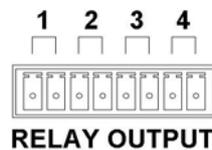
The four low-voltage relay ports are normally open contacts. Each group is independent and isolated, and can bear a load up to 1A 30VAC/DC.
